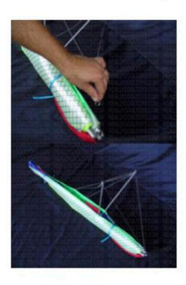
4/ Flip and stand the glider on its control frame and nose and unclip the two remaining buckles.
