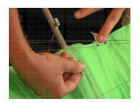
13/ Push down on the keel so that the glider rotates and sits on the control frame and keel.
