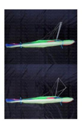
3/ Pull the nose wire ring towards the nose wire retaining bracket and clip into position. (The nose wires should have adequate length to reach the retaining bracket with only a little bit of tension. If they don't, check that the wires are sitting correctly on the nose wire ring, control frame corners and the keel.)
